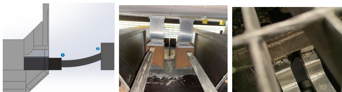
Figure 10. Connection type of aluminium-steel direct welding cathode collector bar for reline cell
