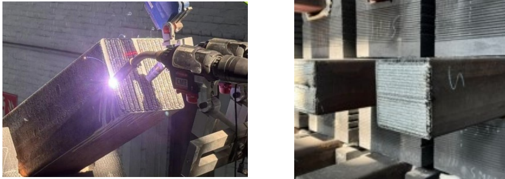
Figure 1. Inclined dual-robotic arm surfacing process for collector bars and resulting weld quality.
